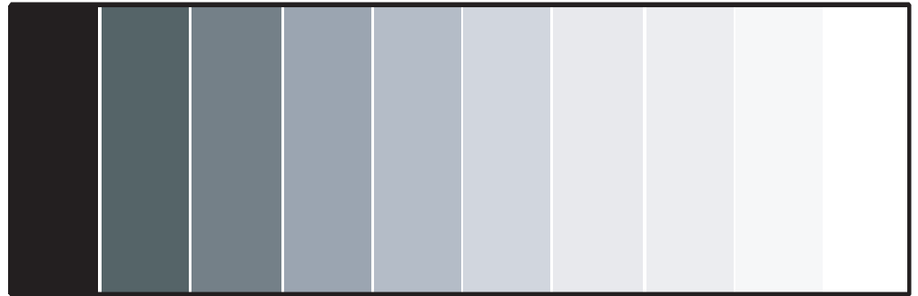
Figure 4-3. Typical Gray Bar Pattern for Adjusting Contrast
